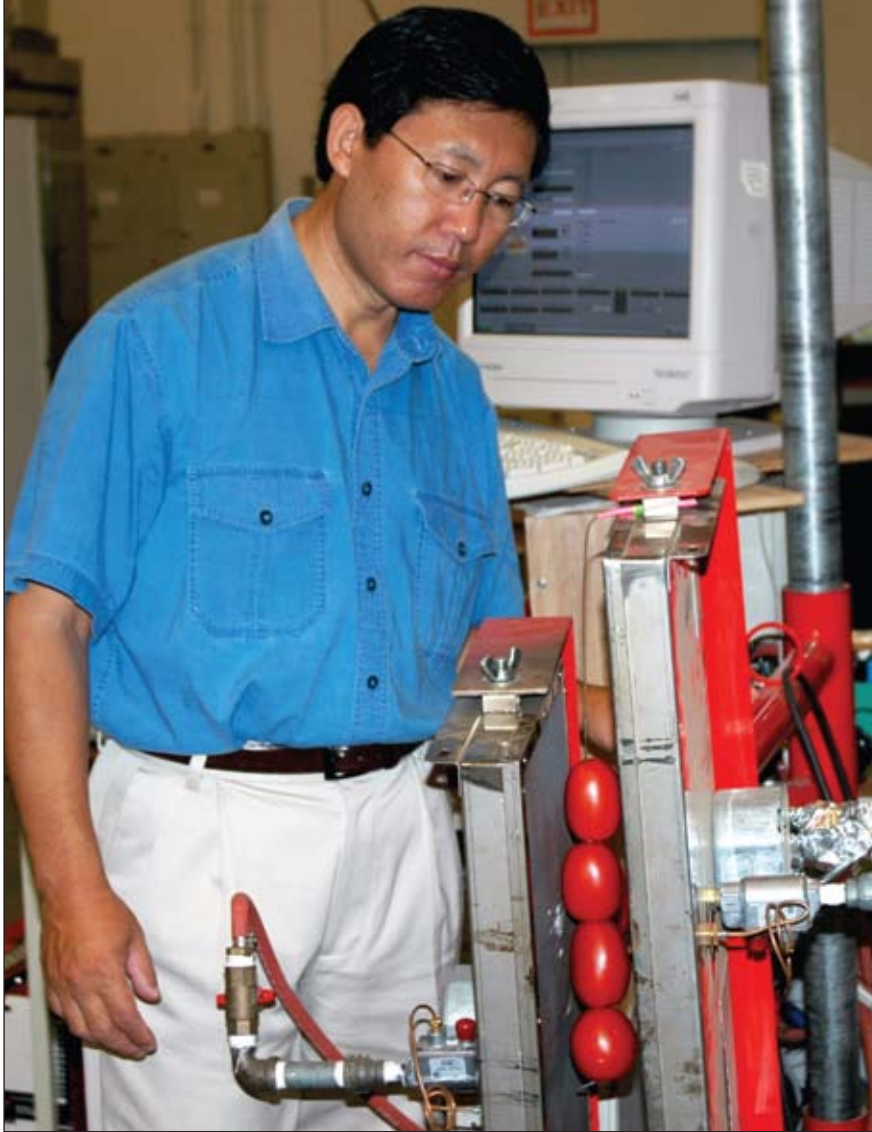
Zhongli Pan, an adjunct professor in the Department of Biological and Agricultural Engineering at UC Davis, treats tomatoes with infrared heat to remove peels prior to processing.
